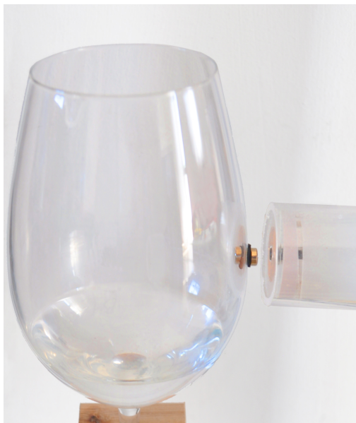
Figure 6: A wine glass fitted with 2 neodymium magnets, one on each side of the glass surface, padded by black foam pads. An electromagnet is placed 2mm away from the outer magnet.
