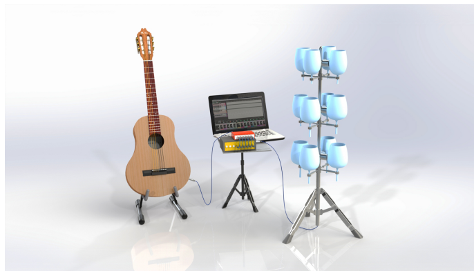
Figure 1: A proposed design of the Symbaline, played by an acoustic guitar, alongside all required system components – Audio interface, Amplification module and PC. (Guitar model: Milos Golijanin, Laptop model: Gopal Kundu).
